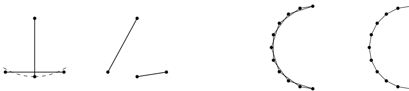
■ Figure 1 Left: A minimum bottleneck matching and a crossing-free minimum bottleneck matching. Right: A minimum bottleneck tour and a minimum bottleneck polygon.
