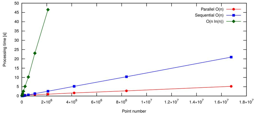
■ **Figure 2** Performance comparison on a multicore architecture.
